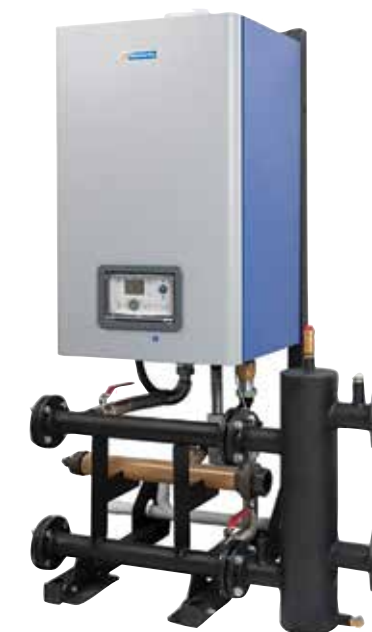
A low loss header ensures adequate flow, resistance and temperature around the primary circuit, while flow rates and temperatures in the secondary circuit may vary.
