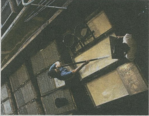
Workers mix raw latex with water and acid in the process of producing rubber sheets at a factory near Khao Chamao village in Rayong province. BLOOMBERG NEWS
